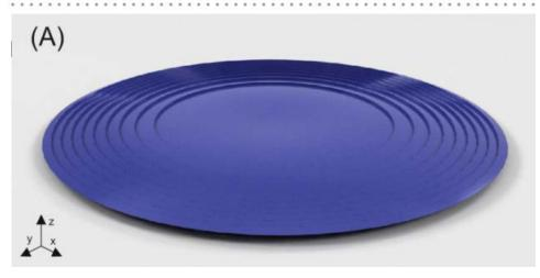
Fresnel-type structures to limit the height of the element
